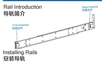
Position the rear bracket and align each pin with the rack holes. Pull the latch release button on the rear bracket. Push the rail into the rack until the square pins are fully seated on the rack holes and the latch clicks into place. 在机柜上确定好导轨后支架的安装位置,将导轨后支架上的方形锁扣和圆形按钮对准机柜角轨上的孔位,参照图中按压后托卡勾,再依图中箭头所示方向推导轨,直到方形锁扣完全卡入角轨孔位。
